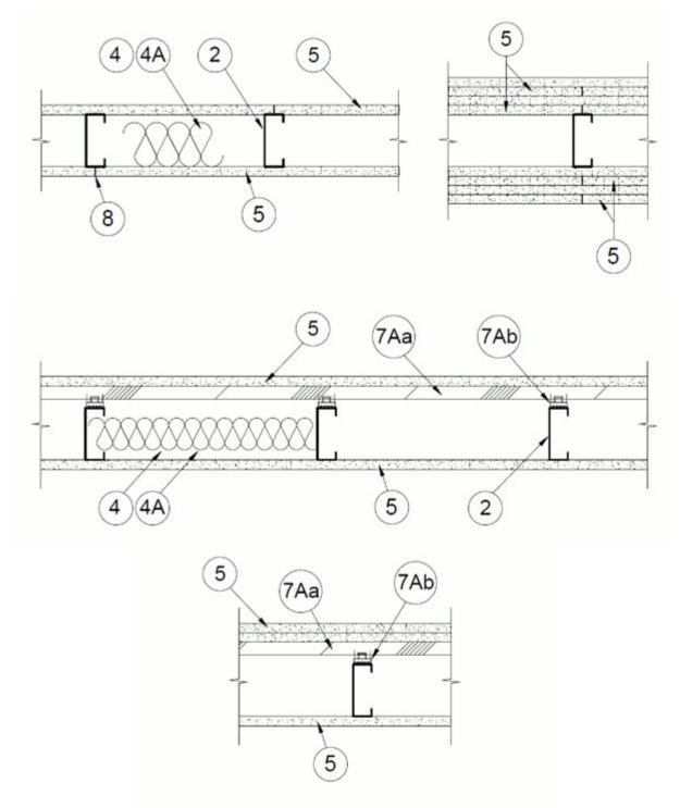
1. Floor and Ceiling Runners — (Not Shown) — For use with Item 2 — Channel shaped, fabricated from min 25 MSG corrosion-protected steel, min depth to accommodate stud size, with min 1-1/4 in. long legs, attached to floor and ceiling with fasteners 24 in. OC max.
